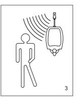
The red light will blink once every 3 seconds when a user is within the detection zone. Initially, the valve flushes for 2 seconds, followed by a 6-second flush after the user exits the area.
